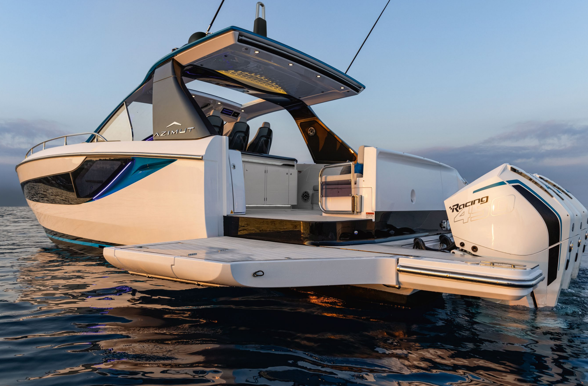
Portside aft bulwark folds out to enlarge the space offering an easy access to the sea.
